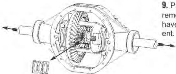
**9.** Pull axles out approx. 8" and remove clutch spring (some may have multiple coil springs) if present.
