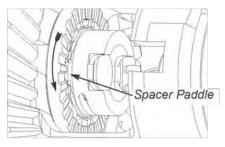
**20.** Insert the non-slotted driver as shown, making sure the paddle opening in driver (missing extended tooth) is facing out towards you.
