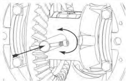
**40.** Using the retaining bolt as a handle, insert the shaft into the differential. Press hard while twisting to pass shaft by springs.
