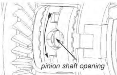
**38.** Feel through pinion shaft opening and verify both spacers and drivers are fully seated onto couplers. Verify all 8 saddle springs are fully seated in holes.
