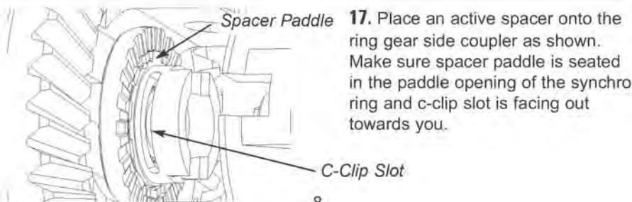
**17.** Place an active spacer onto the ring gear side coupler as shown. Make sure spacer paddle is seated in the paddle opening of the synchro ring and c-clip slot is facing out towards you.
