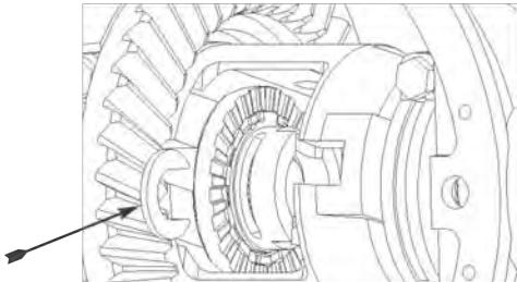
**19.** Rotate ring gear side wheel 1/4 turn back so that the spacer paddle and the opening in the synchro ring are facing out towards you.
