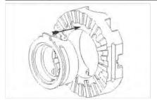
**23.** Insert the second spacer into the slotted driver. Seat the spacer paddle at the paddle opening in the driver (missing extended tooth).
