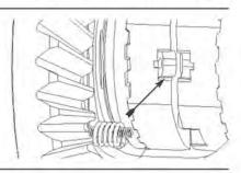
32. Visually inspect notches in spring slot to make sure inner spring is fully seated.
