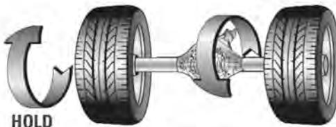
45. After sharply turning the passenger side wheel in the opposite direction (to disengage the unit), the wheel should rotate freely.
