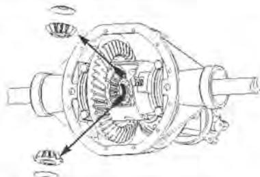
**10.** Remove both spider gears and their thrust washers.
