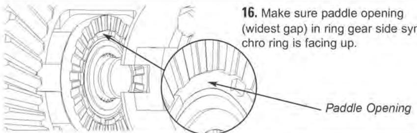
**16.** Make sure paddle opening (widest gap) in ring gear side synchro ring is facing up.
