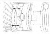
**26.** Wedge both drivers in engagement with couplers. Rotate driver's side wheel forward 1/4 turn to reveal spring slot.
