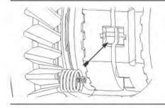
**28.** Compress inner spring and install spring assembly into spring slot.
