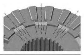
**13.** Apply wheel bearing grease to driver teeth and spacer.
