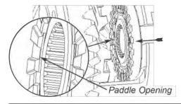
**22.** Insert the second coupler into the differential. Verify paddle opening (widest gap) in other synchro ring is facing away from you.
