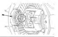
**25.** Verify spacer paddle is aligned with the paddle opening in synchro ring and press down on driver/spacer to seat on coupler; driver teeth should be fully engaged all the way around.
