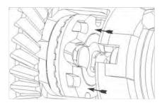
**21.** Press driver down onto coupler. Driver teeth should be fully engaged all the way around.
