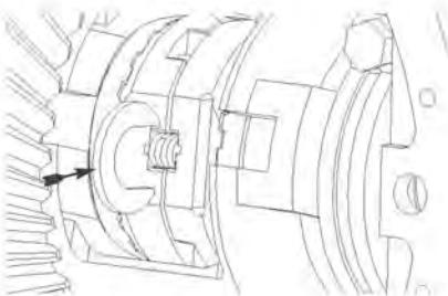
**37.** Making sure drivers stay engaged with couplers, carefully rotate both wheels backwards 1/4 turn to expose pinion shaft opening.
