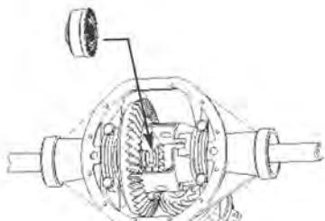
**15.** Install coupler inside ring gear side of differential case.
