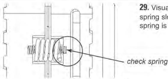
**29.** Visually inspect notches in spring slot to make sure inner spring is fully seated.
