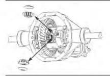
**10.** Remove both spider gears and their thrust washers.
