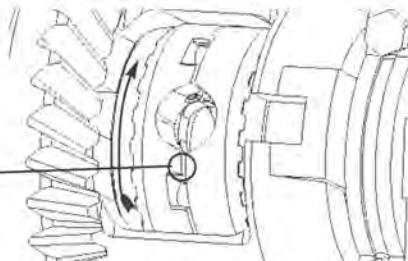
**31.** Compress inner spring and install the second spring assembly into the second spring slot.
