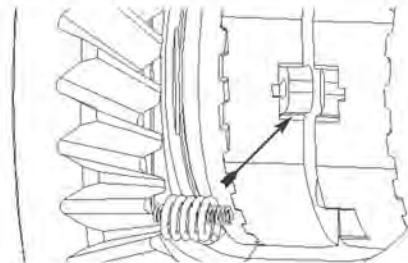
**32.** Visually inspect notches in spring slot to make sure inner spring is fully seated.
