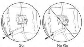
**33.** Check the gap between drivers using check block. The narrow side of the block should fit between the drivers, but the wider side should not fit.
