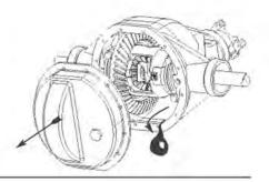
7. Expose pinion shaft;remove retaining bolt and shaft.
