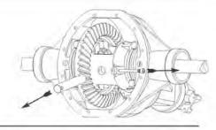
8. Push both axles inward and remove both c-clips. Remove orings from c-clip grooves on axle shafts if present.
