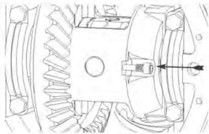
**41.** Insert retaining bolt into case/shaft. Tighten retaining bolt firmly.
