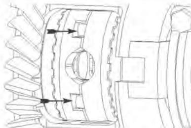
**26.** Wedge both drivers in engagement with couplers. Rotate driver's side wheel forward 1/4 turn to reveal spring slot.
