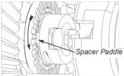
**20.** Insert the non-slotted driver as shown, making sure the paddle opening in driver (missing extended tooth) is facing out towards you.
