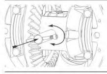
**40.** Using the retaining bolt as a handle, insert the shaft into the differential. Press hard while twisting to pass shaft by springs.
