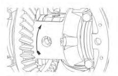
**39.** Keeping couplers and drivers stationary, rotate case 1/4 turn forward to align pinion shaft openings.
