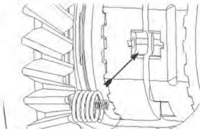
**28.** Compress inner spring and install spring assembly into spring slot.
