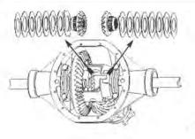
**11.** Remove side gears, clutches, and thrust washers.
