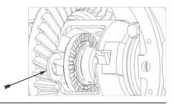
**19.** Rotate ring gear side wheel 1/4 turn back so that the spacer paddle and the opening in the synchro ring are facing out towards you.
